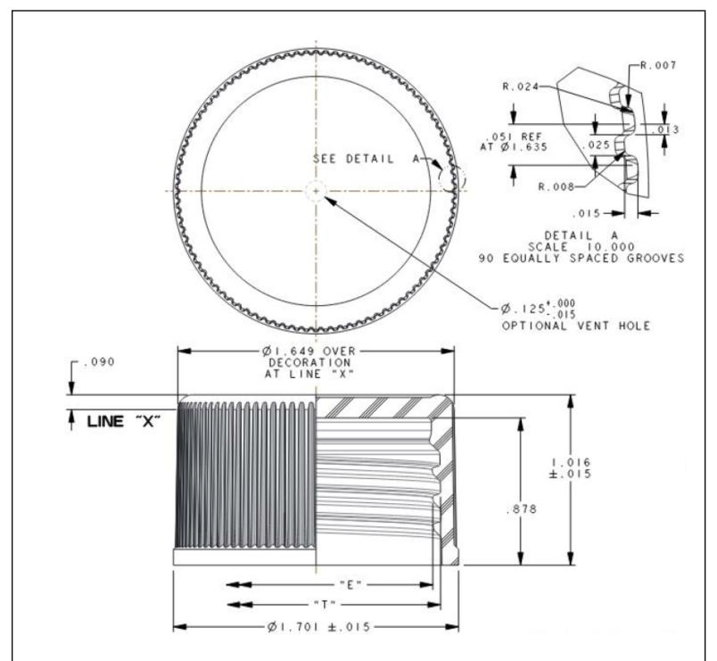
**Description:** 38-439 black polypropylene (PP) closure lined with a polyethylene (PE) core encapsulated between two layers of polyethylene film
